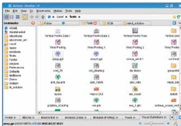
Figure 1 The main window of Metview's new user interface. The central part contains the folder views organised into a set of tabs. To the left there is the bookmarks sidebar, while the folder navigation actions together with clickable folder location bar are located in the toolbar at the top. The bottom part of the desktop, just like in the previous user interface, is occupied by the icon drawers. The status bar, at the very bottom of the desktop, displays useful information about the icon that the mouse cursor currently hovers over.
