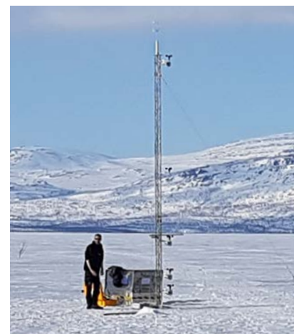
Fieldwork on a frozen lake. Micrometeorological mast installed on Lake Torneträsk.
