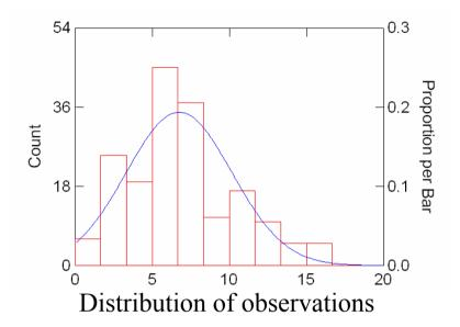
Error distribution of EPS mean forecasts (sample of 180 cases) and fitted Gaussian distribution BLUE line corresponds to mean spread of EPS mean
