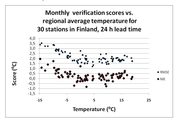
Picture 1. The result demonstrates linear dependence of forecast accuracy on surface air temperature at below  $0\,^{\rm 0}{\rm C}$  conditions
