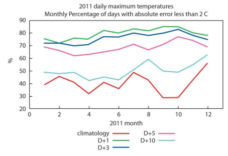
*Figure 1.* Time series of percentage of correct maximum temperature forecasts (error less than 2°C) for different prediction ranges. The verification sample is composed by the forecasts made in 2011 for a set of 50 Spanish synoptic stations.
