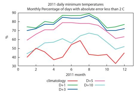
**Figure 3.** Time series of percentage of correct minimum temperature forecasts (error less than 2°C) for different prediction ranges. The verification sample is composed by the forecasts made in 2011 for a set of 50 Spanish synoptic stations.
